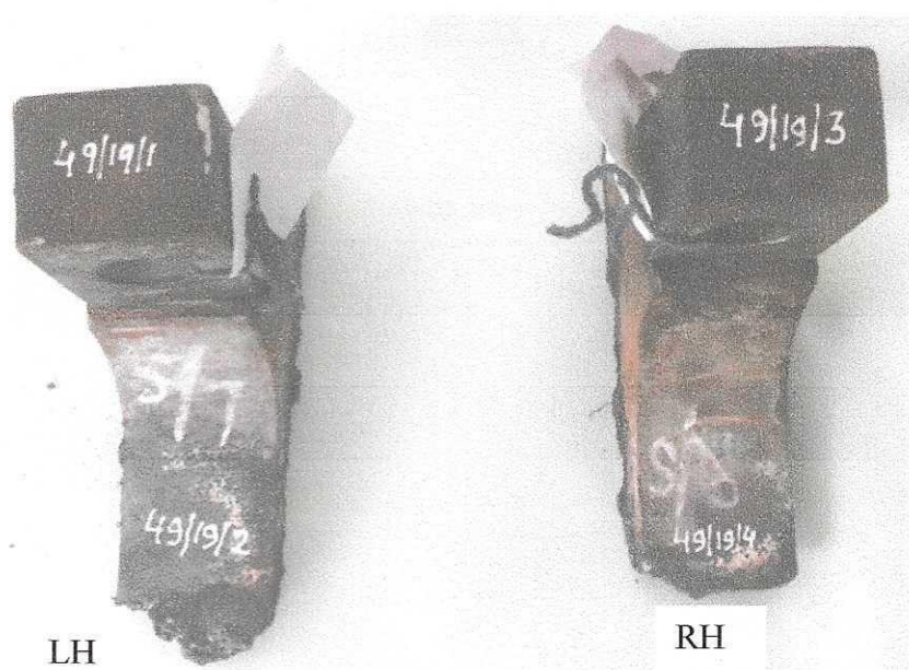
Fig.1: Photograph showing fractured LH & RH side traction motor-3 support lug pieces in as received condition.
